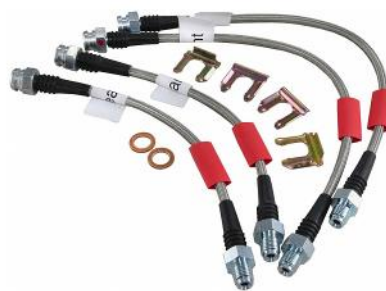
1002208 Brake Hose Set, Braided Stainless Steel, 1963-1982 ..... 157.99
